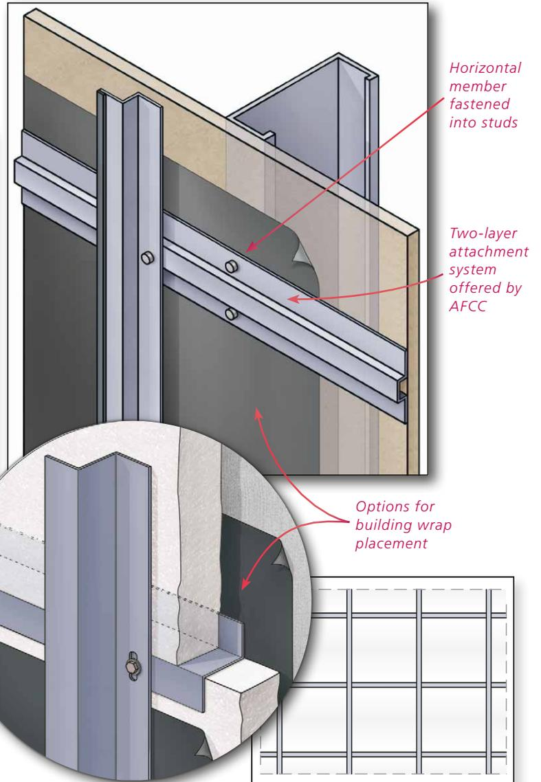
**FIG. D-2** — Exterior insulation, when vertical profiles are attached to horizontal profiles affixed to wall.
