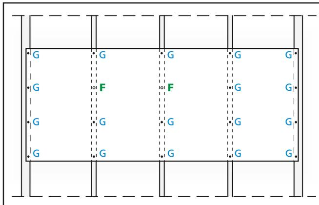
▼ *FIG. G* — Horizontal installation on vertical profiles
