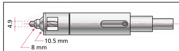
For centering pilot hole in profile for **Fixed Points** and **Gliding Points**.
