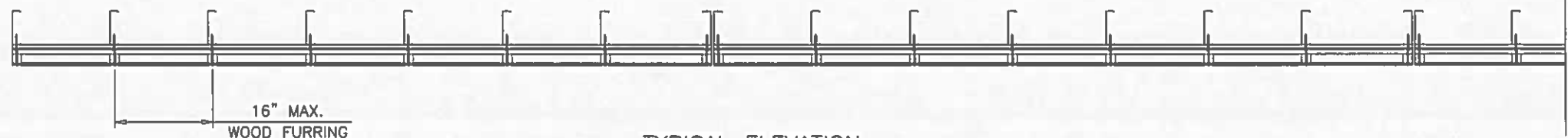
TYPICAL ELEVATION INSTALLATION AT STEEL STUD FRAMING SYSTEM USING 2X2 WOOD FURRING & 'Z' CLIPS
