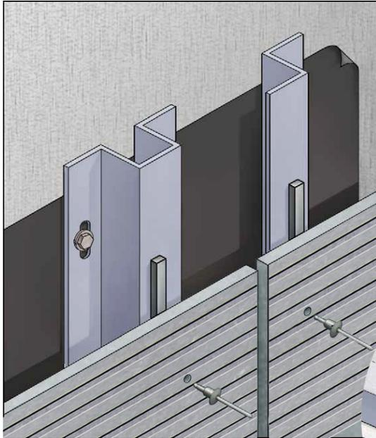
Hat channel can be attached with the crown facing in or out, depending on fastener spacing and the visibility of the profile through the joint.
