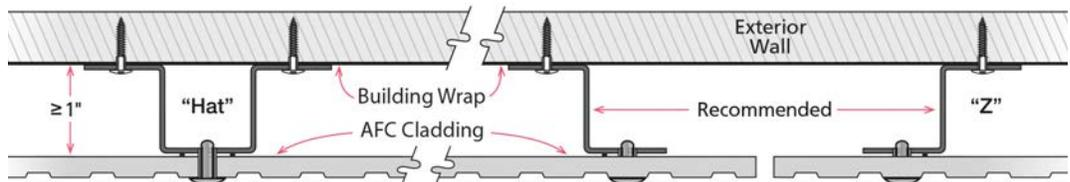
Can be vertically affixed directly to wall if there is no exterior insulation, provided sheathing has adequate screw-holding strength; (3/4" plywood sheathing is recommended).
